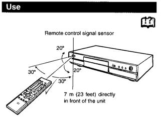
Aim at the sensor, avoiding obstacles, at a maximum range of 7 m (23 feet) directly in front of the unit.
